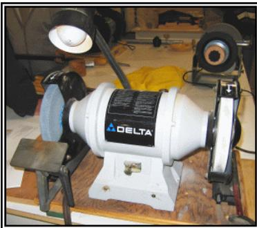
Our demonstration last month was a good one. Jim Talley brought his One Way Wolverine Sharpening system, and gave us some basic pointers on sharpening. The Wolverine system consists of a Delta Grinder with a couple
