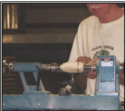
The egg is beginning to take shape. Notice the turned flange on the right end of the blank. This will be mounted in a chuck to enable parting off the small end.
