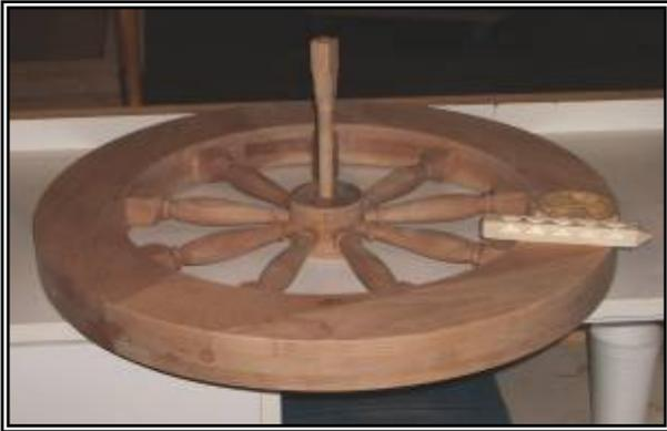
Shown here is a good start on my treadle lathe. The flywheel is the most difficult part and the most interesting to me. The best part was building all the jigs to get all the parts concentric. I also learned a great deal about using a skew chisel on these nine spindles and the hub. Not shown are the other three spindles that I *really* messed up!
