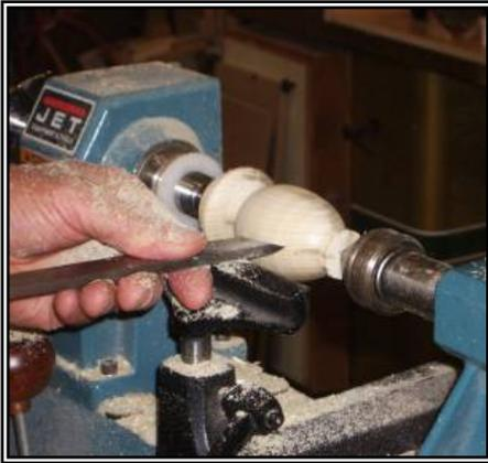
Here you can see the egg taking on the final shape before the sanding and finishing. Michael finishes his eggs on the lathe using a spray lacquer and a buffing rag. After the finishing, the flange on the left hand end of the blank will be mounted in the chuck and the small end parted off. I don't have a photo of this step.
