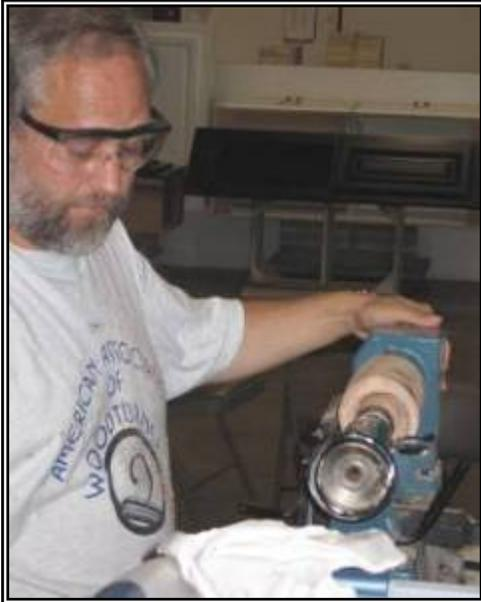
Rodney starts by turning the blank between centers, cutting a tenon on the base, and shaping the mouth.
