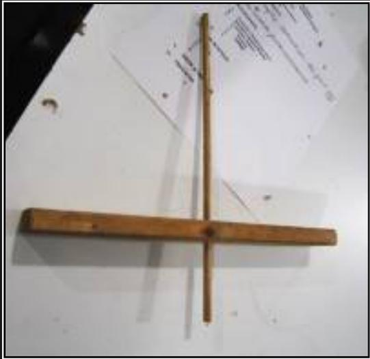
Here is Rodney's homemade depth gauge to help prevent making the inside larger than the outside! You can just see the bolt used to hold the dowel in place once you get it set to the desired depth.
