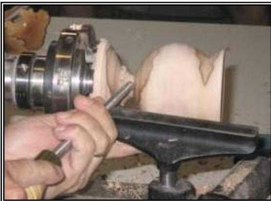
On this point the outside has been shaped, the inside has been hollowed and all has been sanded to perfection. Then you must part off the piece to begin the final shaping and sanding of the bottom.
