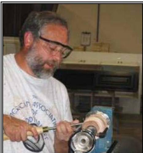
The next step is to chuck up the base tenon and shape the main body of the vessel.
