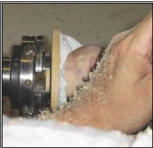
Here the bowl is being fitted to the jamb chuck with a paper towel to take up the clearance. Once this is fitted, you can clean up the bottom.
