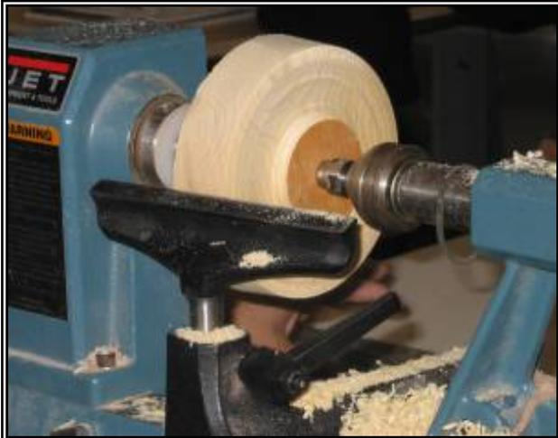
Here one must create a jamb chuck so as to be able to reverse the pot for the final finishing. A jamb chuck is a shape that will fit inside the vessel fairly tightly to hold it while finishing up the area that was parted off. If it is made a tad too small, then you can always wrap paper around it to tighten up the fit.
