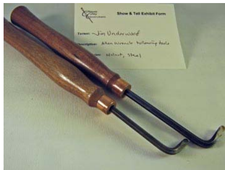
Allan wrench hollowing tools made by Jim Underwood
