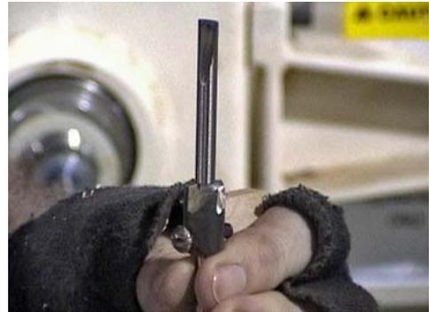
The fourth "tool" consists of the appropriate bushings for the pen kit. In many cases the 7 mm drill and 7 mm bushings will come with a mandrel as a "kit". Slimline kits, which are the most popular kits, use this drill and these bushings.
