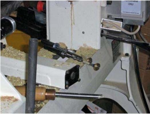
is probably the standard mandrel. The shaft is easily replaceable and inexpensive. An adjustable shaft mandrel is also available, and its shaft is replaceable too. The advantage of this model is that you do not have to supply more bushings if the pen kit is smaller than normal, you simply adjust the shaft to the shorter size.
