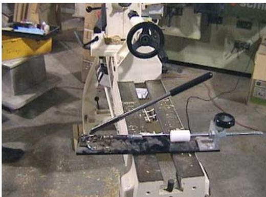
Once the pen blanks have been turned and finished the only thing left to do is to assemble the pen blanks. You can use a variety of methods to press the parts together, such as a large vise, clamps, drill press, arbor press or pen press purchased from a supply catalog or store. There are also plans available on the Internet for building pen presses.
