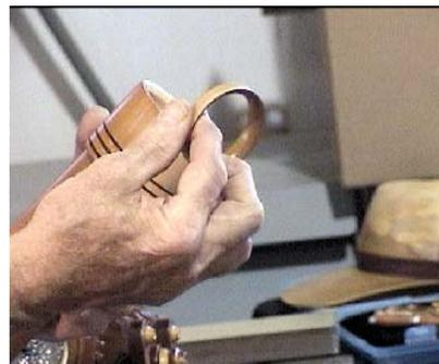
The final assembly step involves securing the rotating barrel end to the central cylinder using retaining washers and screws into the tenon end, inserting the object box and turning a wooden retaining ring to hold this in place.
